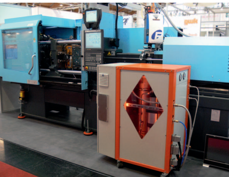
Fig. 7. The installation for dynamic mold temperature control combines rapid heating and cooling changes at temperature gradients of up to 20 K s -1 (photo: gwk)
